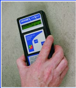
% Moisture Concrete Slab
